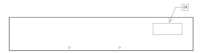
19. <u>AC POWER INPUT</u>. A three-pronged recessed male connector is provided on the back panel for AC power connection to the instrument. Also contained in this assembly is a slow blow fuse and a removable card that can be removed and repositioned to switch between 120V AC in and 240V AC in.
